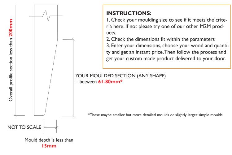
You can use this custom profile for any product that is produced as a linear moulding where the general characteristics of your profile fall within the guidelines shown.
